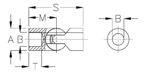
A = 90 B H7 = 60 M = 130.0 Max torque (Nm) = 1060 s = 260 T = 70
